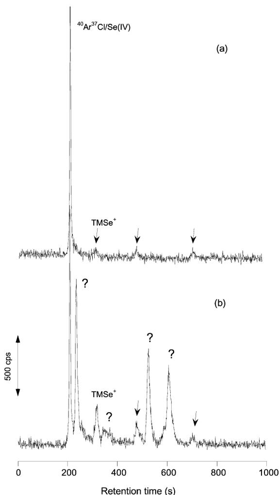
**Fig. 3** Chromatograms of the urine reference material (NIST SRM 2670): (a) normal level; (b) elevated level. The Se isotope  $m/z$  77 was monitored by ICP-MS.
