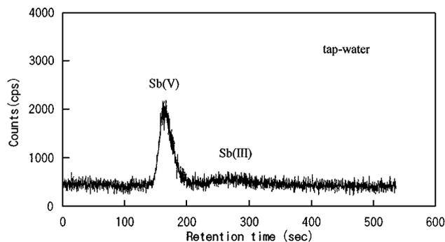
Fig. 2 Chromatogram for the determination of Sb species in a tap-water sample. Chromatographic conditions as in Fig. 1.
