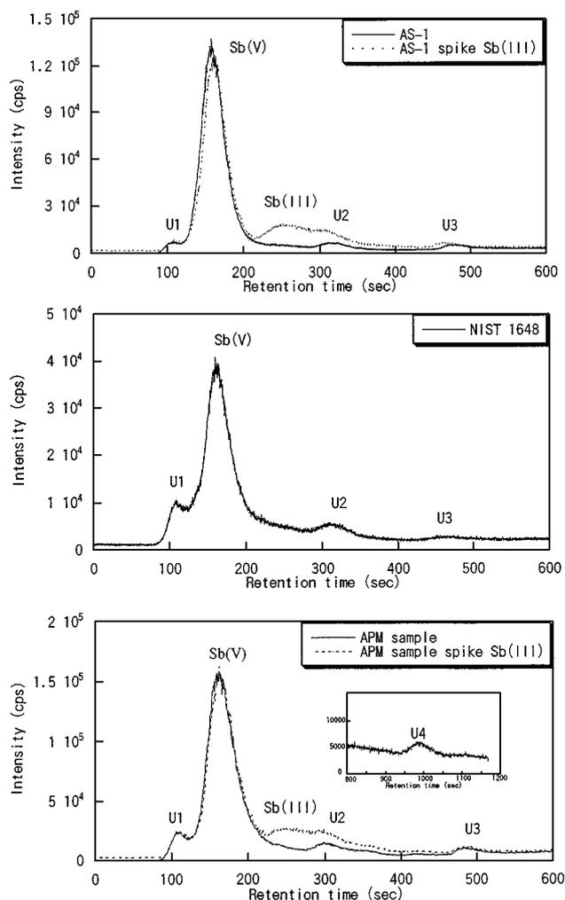
Fig. 3 Chromatograms resulting from the analysis of the aqueous extracts of airborne particulate matter: a Japanese quality control sample (AS-1), a standard reference material (NIST 1648), and a sample collected in Tokyo (APM sample). The chromatographic conditions are as in Fig. 1. The dotted lines indicate chromatograms obtained after spiking Sb(III) standard (50  $\mu\text{g/l}$ ) into the extracts of AS-1 and APM sample.
