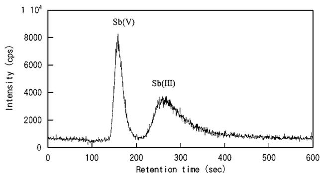
Fig. 1 Chromatogram of the separation of Sb(III) and Sb(V) ( $5 \mu\text{g/l}$  Sb, each) on Synchropak Q300 column. Mobile phase: 2 mmol/l phthalic acid-5 mmol/l EDTA, pH 4.5; Flow rate: 1.0 ml/min; Detection: ICP-MS at mass 121. The summation of integrated signals of Sb(V) and Sb(III) is 32000 counts and 34300 counts, respectively.
