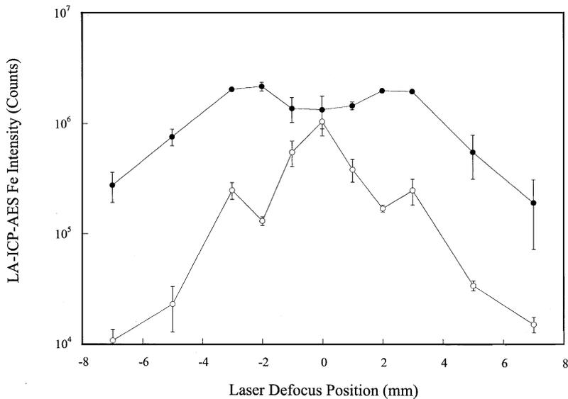
Fig. 8. LA-ICP-AES Fe I 373.5 nm intensities for low-alloy steel and pond sediment as a function of laser defocus position. Low-alloy steel (—○—), pond sediment pellet (—●—). Error bars indicate  $\pm 1$  SD ( $n=3$ ).
