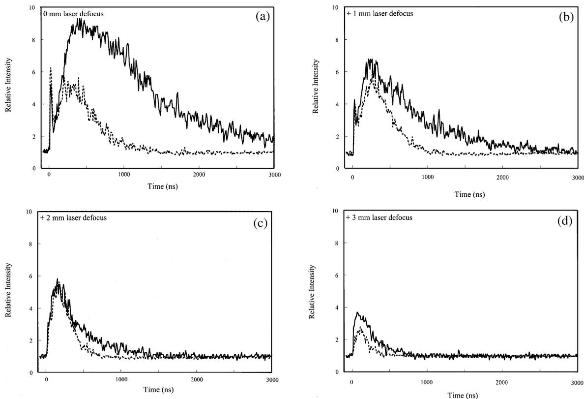
Fig. 5. (a) Relative LIP Fe intensities for the low-alloy steel and pond sediment pellet in-focus laser position. Low-alloy steel (—), pond sediment pellet (----). (b) As in (a) +1 mm laser defocus position. (c) As in (a) +2 mm laser defocus position. (d) As in (a) +3 mm laser defocus position.
