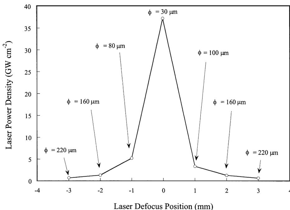
Fig. 2. Estimated laser power density of the LA system as a function of laser defocus position. This was estimated using a certified low-alloy steel sample. Crater diameters for each laser defocus position are also indicated. The laser output energy was constant at  $2.1 \pm 0.1$  mJ during all experiments.
