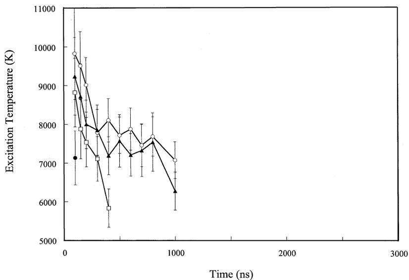
Fig. 7. LIP  $T_{\text{ex}}$  for different laser defocus positions for pond sediment pellet. 0 mm (—○—); +1 mm (—▲—); +2 mm (—□—); +3 mm (—●—). Error bars indicate  $\pm 1$  SD calculated from the deviation from a linear regression curve of a Boltzmann plot.
