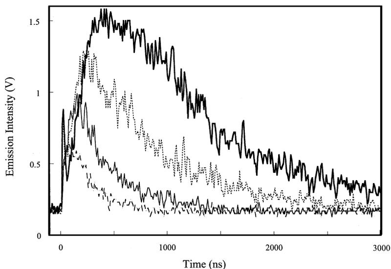
Fig. 3. LIP Fe I 373.5 nm emission signals for in-focus and positive laser defocus positions for low-alloy steel. 0 mm (—); +1 mm (----); +2 mm (— · —); +3 mm (· · ·). LIP Fe emission signals were measured using a PMT. The high voltage was  $-500$  V during these measurements.
