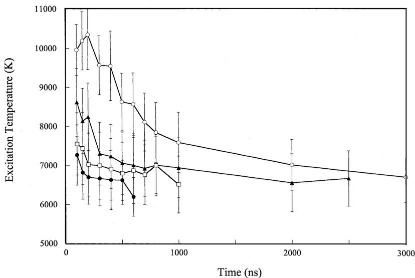
Fig. 6. LIP  $T_{\text{ex}}$  for different laser defocus positions for low-alloy steel. 0 mm (—○—); +1 mm (—▲—); +2 mm (—□—); +3 mm (—●—). Error bars indicate  $\pm 1$  SD calculated from the deviation from a linear regression curve of a Boltzmann plot.
