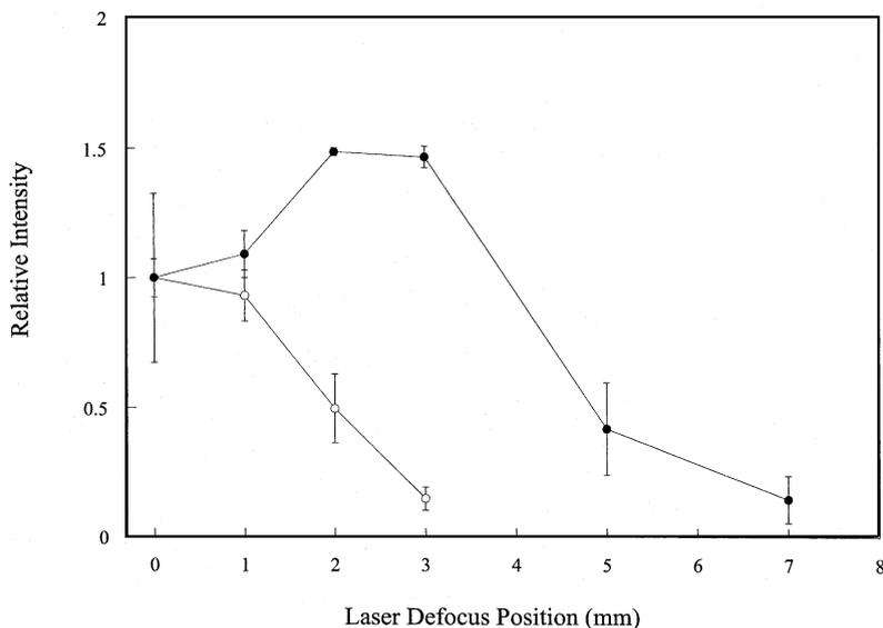
Fig. 10. Relative Fe intensities for LIP Fe and LA-ICP-AES for pond sediment as a function of laser defocus position. LIP Fe (○), LA-ICP-AES Fe (●). Error bars indicate  $\pm 1$  SD ( $n=3$ ).
