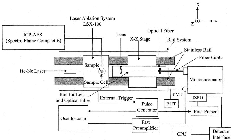
Fig. 1. Schematic diagram of the instrument configuration used for measuring LIP emission and LA-ICP-AES.
