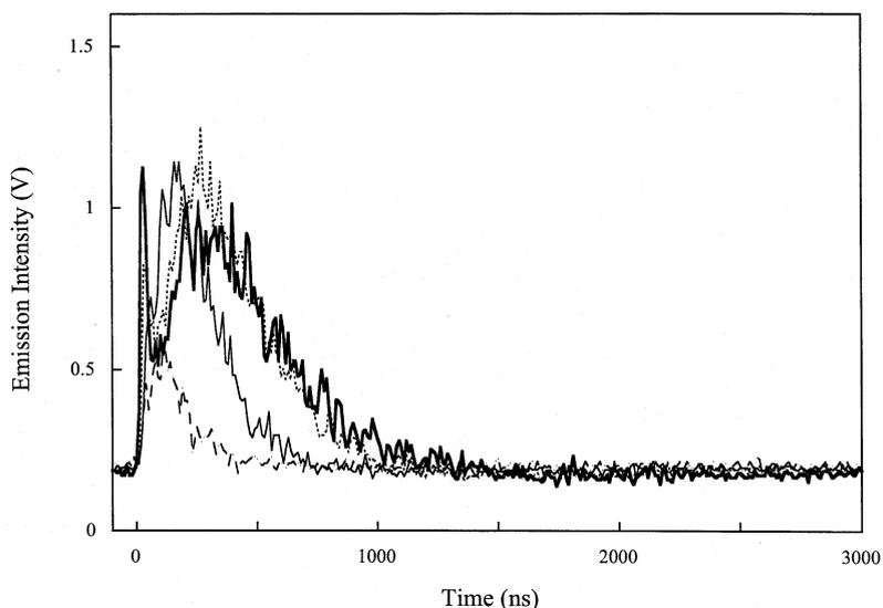
Fig. 4. LIP Fe I 373.5 nm emission signals for in-focus and positive laser defocus positions for NIES pond sediment pellet. 0 mm (—); +1 mm (----); +2 mm (— · —); +3 mm (· · ·). LIP Fe emission signals were measured using a PMT. The high voltage was  $-600$  V during these measurements.
