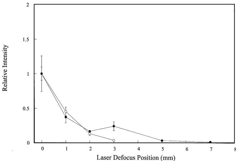
Fig. 9. Relative Fe intensities for LIP and LA-ICP-AES for low-alloy steel as a function of laser defocus position. LIP Fe (—○—), LA-ICP-AES Fe (—●—). Error bars indicate  $\pm 1$  SD ( $n=3$ ).
